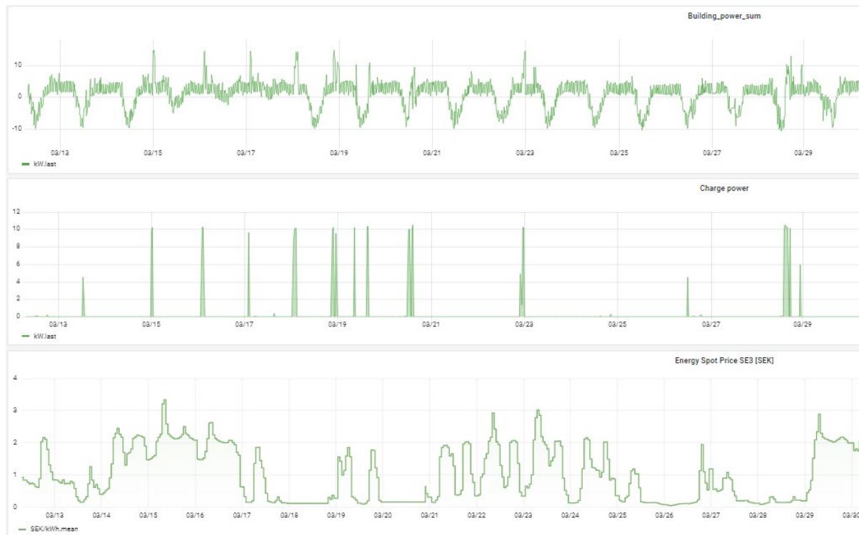
Figure 3: Optimiser results (Nordpool 2 SE3 3 ) for a household with solar production. Top figure shows the dynamic power delivered to the household. Middle figure shows the charging occasions considering the lowest price tariff. Bottom figure shows the price tariff (Nordpool SE3).
