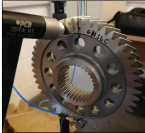
Figure 9: Gear Modal Testing
