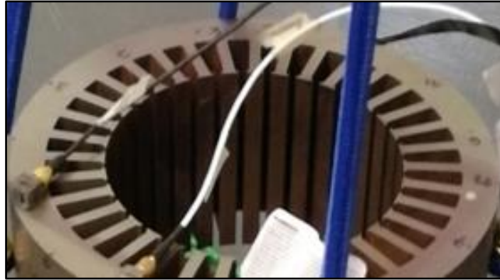
Figure 4: Stator Lamination Stack
