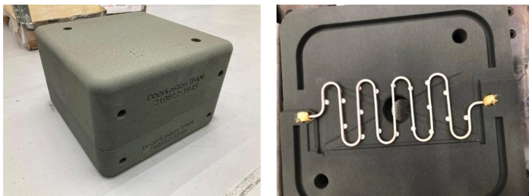
Figure 4: Core package made of 3D-printed sand, in two parts. Left: Top and bottom box assembled; Right: Copper cooling channel positioned in the bottom box with the help of core blocks.
