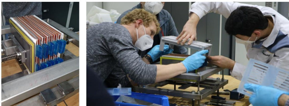
Figure 9: Demonstrator assembly: left: Positioning of the cell stack in the joining device; right: Assembly of the module shells.
