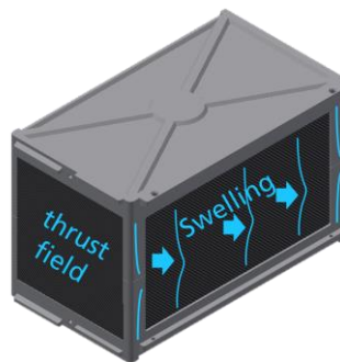
Figure 7: Load case "Internal pressure as a result of swelling of the punched cell stack during loading".
