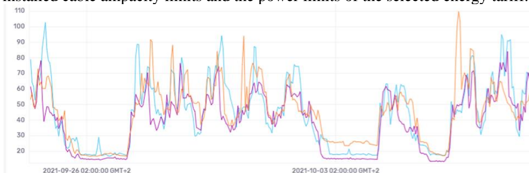
Figure 7: Parcel delivery site#1 in operation: 3-phase currents (A) at the main breaker
