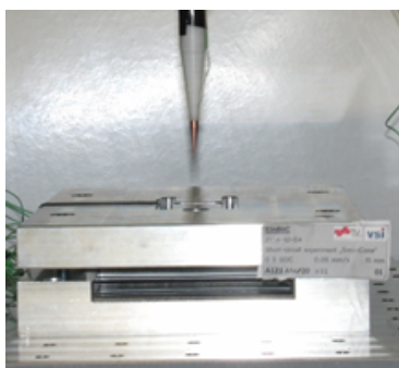
Figure 27: Test situation for "Smart-Cone" cell penetration tests.
