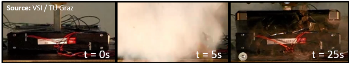
Figure 33: Exothermic reaction during module test no. 2
