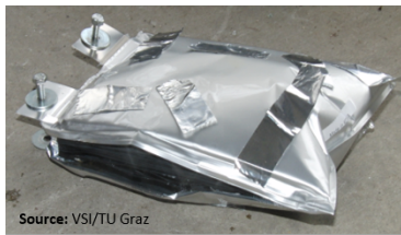
Figure 25: Specimen after high temperature exposure (> 100 °C).
