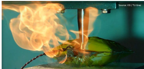
Figure 1: Puncture penetration test with pouch-type Li-ion cell.
