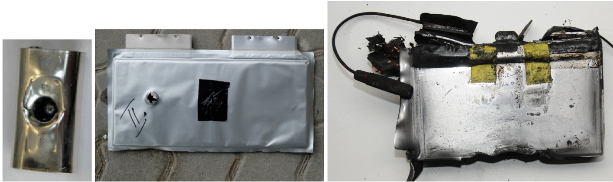
Figure 4: Post-test photographs of cells. From left to right: elliptical cell, pouch cell B and prismatic cell. The prismatic cell was tested with SOC = 100%, the other two cells with SOC = 0%.
