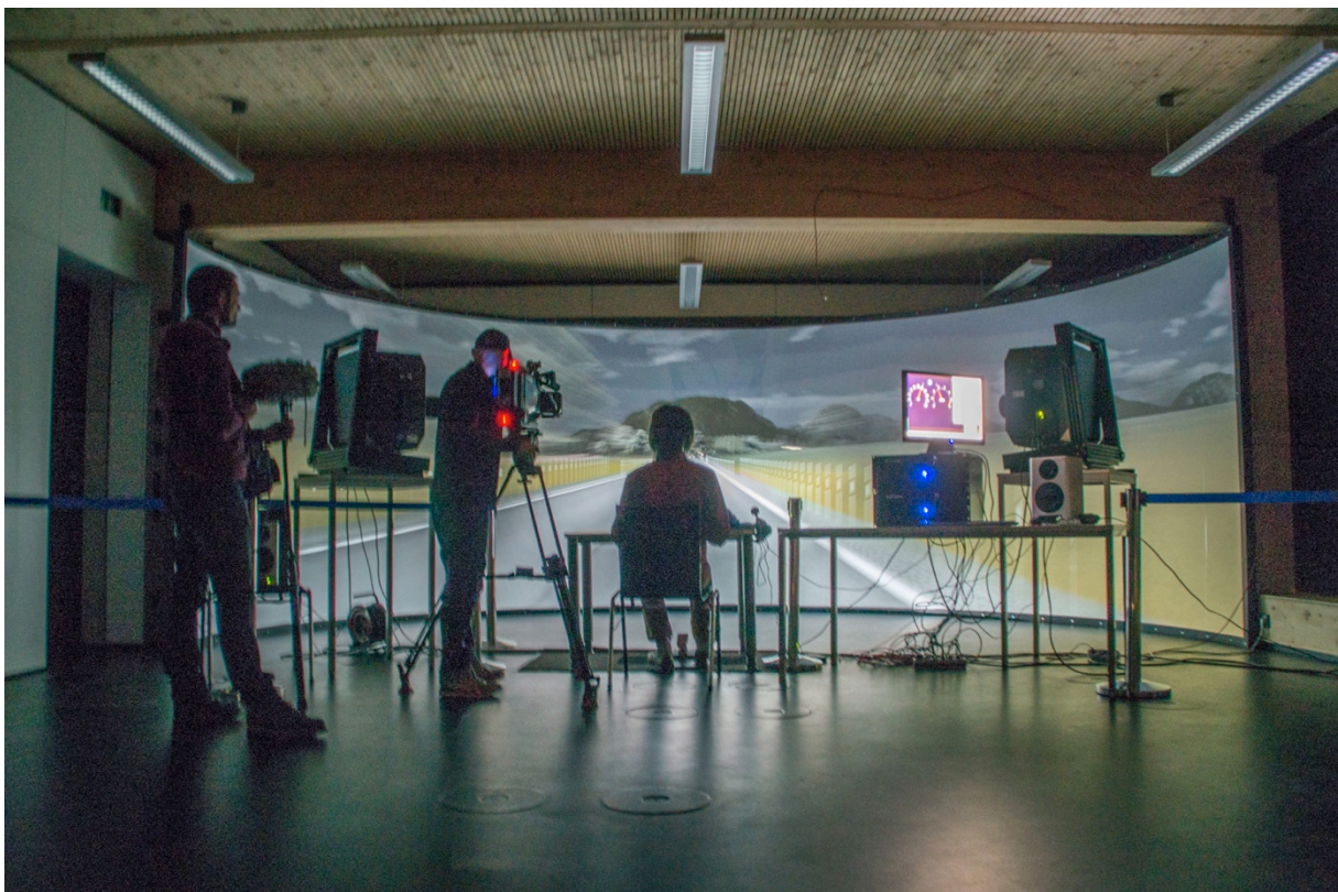
Figure 1: Nighttime driving scenario in the driving simulator of the Aalen Mobility Perception & Exploration Laboratory (AMPEL), created by two high performance projecting units (Velvet 1600, ZEISS Inc., Jena/FRG) illuminating a cylindrical screen in crosswise projection
