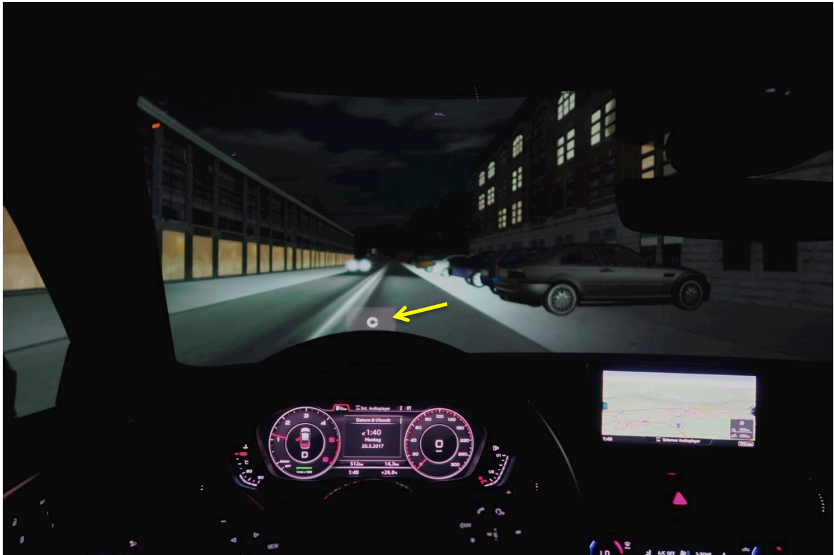
Figure 2: Approaching vehicle under virtual reality nighttime driving conditions in the AMPEL lab: A close-to reality glare simulation cannot be achieved within the usual projecting setting: The two headlights of the approaching vehicle are no more than two white circular areas that do not induce any glare sensation. The yellow arrow points to an optotype (LANDOLT C) which is presented via the modified Head up Display (HUD) of the car for dynamic assessment of visual acuity
