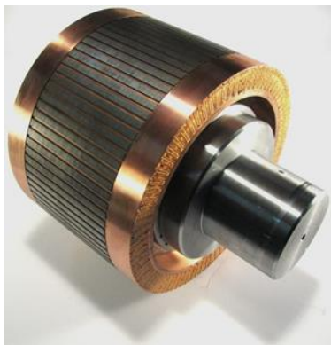
Fig. 2. Axially laser welded copper rotor.
