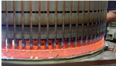
Fig. 1. Induction brazing process.
