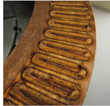
Fig. 3. Axially laser welded copper bars in end ring.
