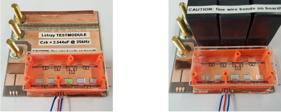
Figure 2: LinkPack test modules equipped with 2.5 \mu\text{F} ceramic capacitors (left) and 45 \mu\text{F} film capacitors (right).
