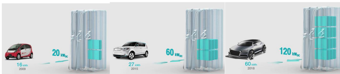
Picture 1: upgradeability of a Multi-Charger for remaining futureproof (EVTEC Switzerland, 2015)
