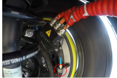
Figure 14: Accelerometer positioning on the stator of the M700 in-wheel motor
