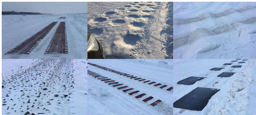
Figure 12: Examples of testing surfaces: Belgian block road, potholes, waves, embedded rocks, bricks, speed bumps
