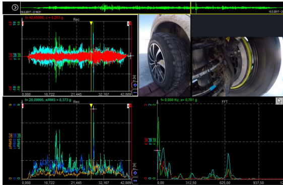
Figure 15: Online analysis of the stator vibrations
