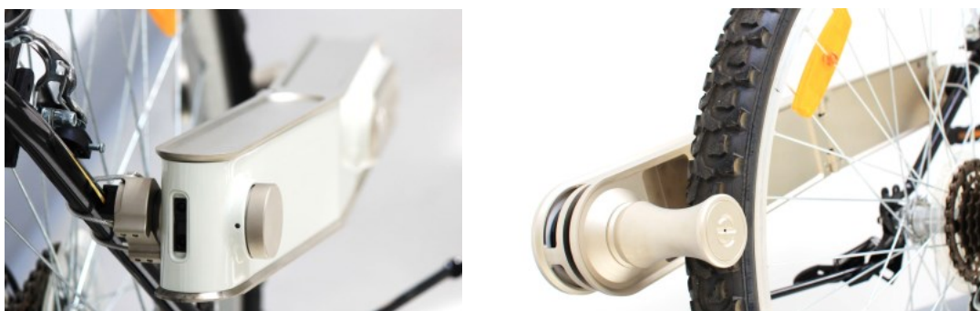
Figure 2(a): Mounting and proximity sensor; Figure 2(b): Friction roller engagement
