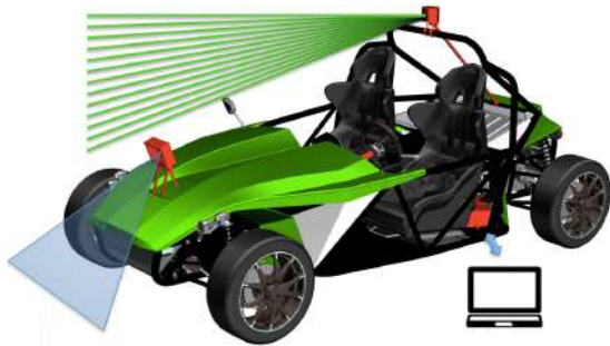
Figure 1: An illustration of our Autonomous eRod. The sensors, actuators and computer providing autonomous driving functionalities are shown in red.
