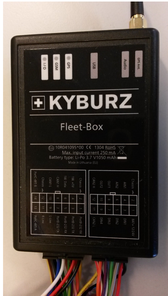
Figure 2: The Kyburz Fleet Management telematics system, with integrated GSM,GPS,CAN, and motion modules
