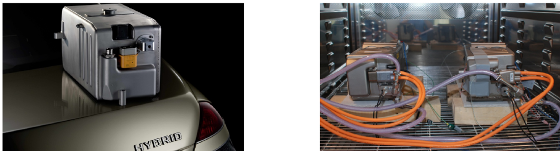
Figure 3: The Mercedes-Benz S400 Hybrid battery (left) and the same battery type in a durability test on the right
