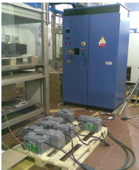
Figure 1: Experimental set-up used for the experimentation. In the foreground is possible to observe the battery packs used for cycle life evaluation
