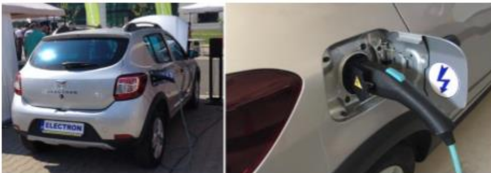
Figure 9: The conductive charging system with home WALL BOX or public station
