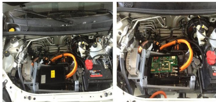
Figure 6: The medium level of the AMBRA powertrain with the Traction Inverter Module TIM 400 type from MES SA
