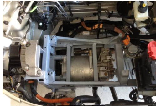
Figure 7: The low level of the AMBRA powertrain with the Electric Motor and Transmission Unit
