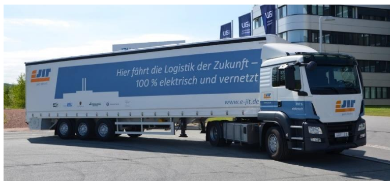
Figure 5: Electric 40t-truck for automotive component delivery at Saxon plants of Volkswagen and Porsche
