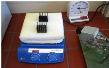
Picture 2: Experimental setup of heat sink comparison
