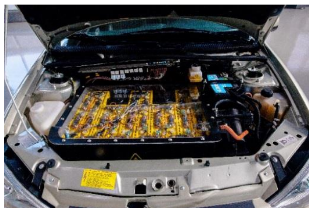
Figure 4: Front block traction batteries with a thermostating system
