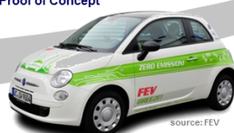
Figure 2: Project BREEZE: Development of a fuel cell plug-in hybrid demonstrator
