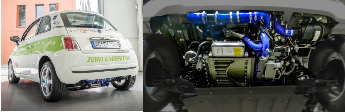
Figure 3: BREEZE demonstrator vehicle and fuel cell system integration (source: ZBT/FEV [6])
