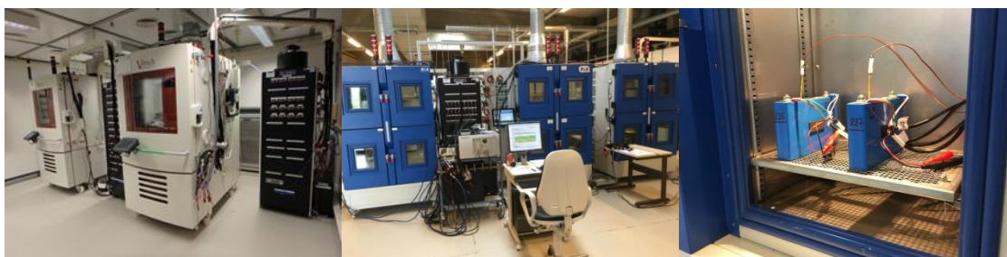
Figure 5: Battery test rigs: Environmental chambers and cyclers (left-centre); Closer view of EV cells under testing inside the environmental chamber (right)
