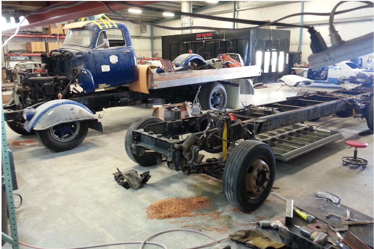
Figure 6: The body from the 1954 GMC is placed onto the modern GMC chassis
