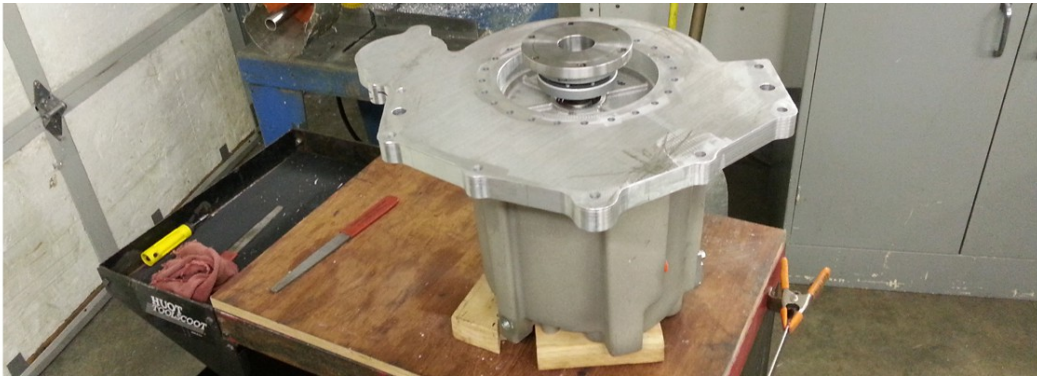
Figure 4: Remy HVH-250 motor with adapter for Eaton Transmission
