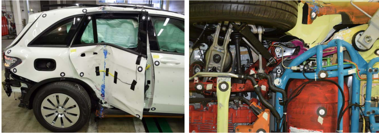
Figure 8: 90° Pole tests according to FMVSS 201 with increased velocity up to 32 km/h instead of 29 km/h
