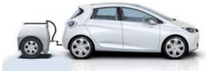
Figure 1: the combination of a Renault Zoe and the EP Tender trailer [20]
