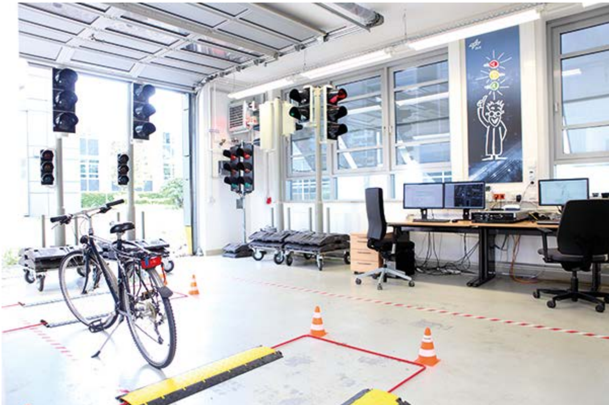
Figure3: LSA-Lab - traffic signal control and engineering in the German Aerospace Center (DLR)
