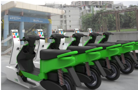
Figure 5 Automatically clamping and charging system
