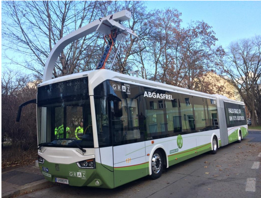
Figure1: Electric bus at charging station in Graz (Source: Graz Holding Linien)
