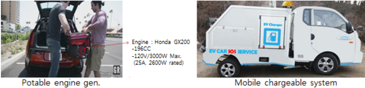
Figure1: Charging method when EV is full discharged. (Potable engine Generator, mobile chargeable system)
