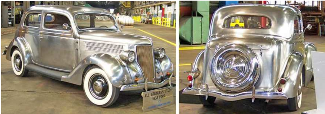
Figure 1: Ford Sedan Deluxe with stainless steel patina after more than 80 years component lifetime [2]
