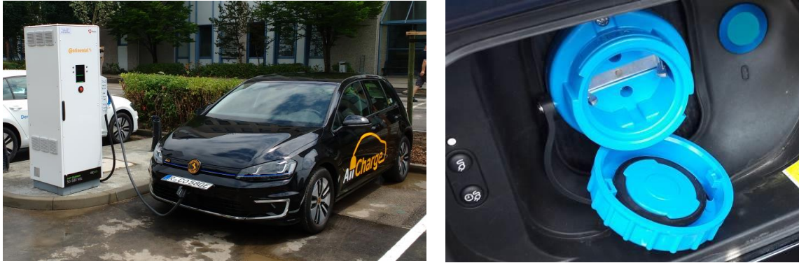
Figure 10: AllCharge demo car / Vehicle-2-Device outlet at former fuel intake
