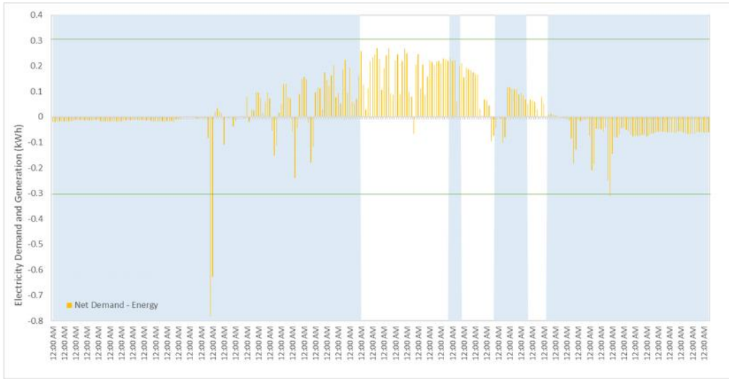
Figure 6: Indication of vehicle availability for V2G services for typical weekday overlaid onto stacked bar chart of property demand and PV generation profile. Also shown is the maximum charge/ discharge converter rates for the V2G unit.
