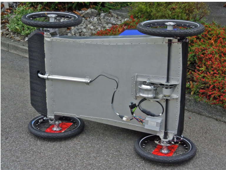
Fig. 2 Platform with integrated Ebike motor and chain to differential
