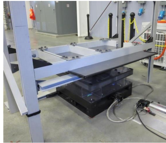
Figure 2. INL's SAE J2954 WPT bench test fixture and test equipment
