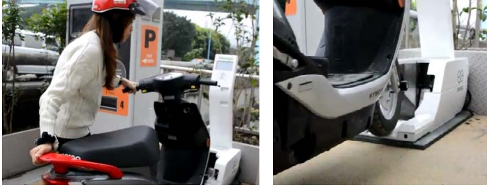
Figure1: Automatic Energy Supply Docking System for E-Scooter
