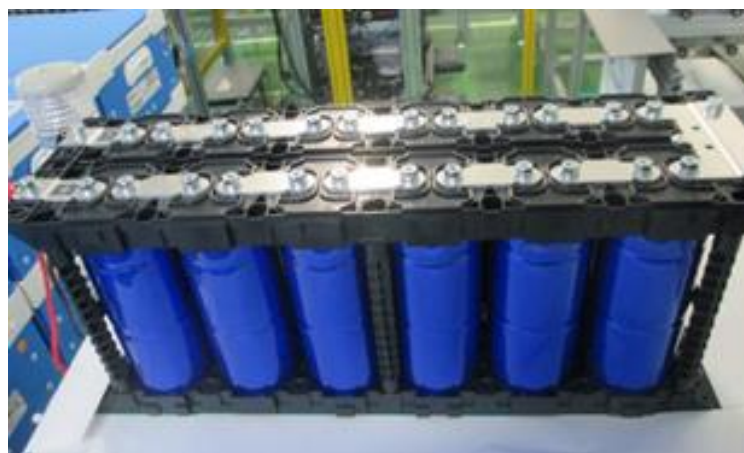
Figure 2: Electrochemical capacitor module used to power the AGV shown in Figure 1. Twelve model DXE 3600-F Nippon Chemi-Con electrochemical capacitors are connected in series. The module is rated at 30 V and can deliver ~100 kJ (28 Wh) with discharge to 15 V.
