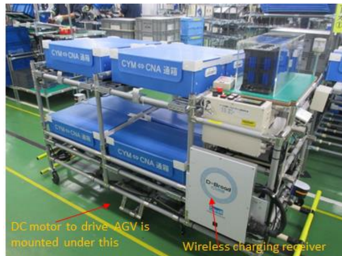
Figure 1: Photograph of capacitor-powered AGV located at the Nippon Chemi-Con factory in Nagaoka, Japan.
