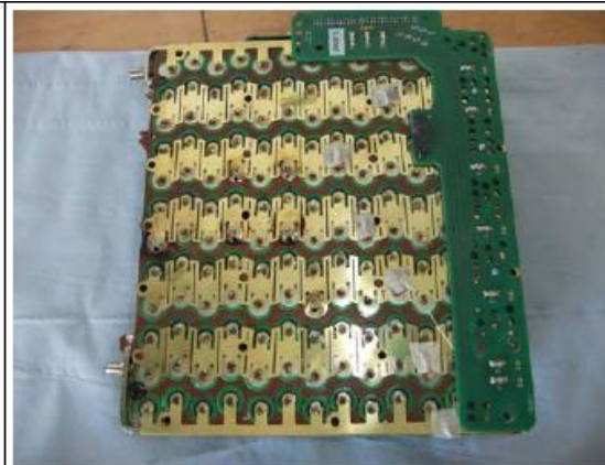
Top view of the module after 6 nail tests
