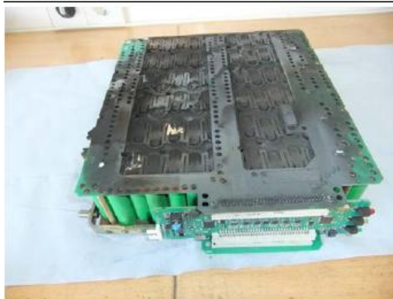
Bottom view of the module after 6 nail tests
