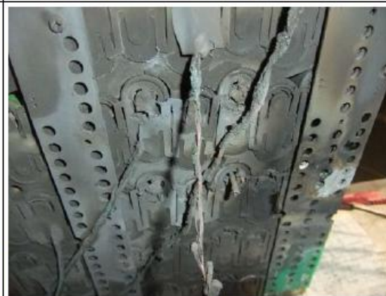
Detailed bottom view of the module after 6 nail tests
