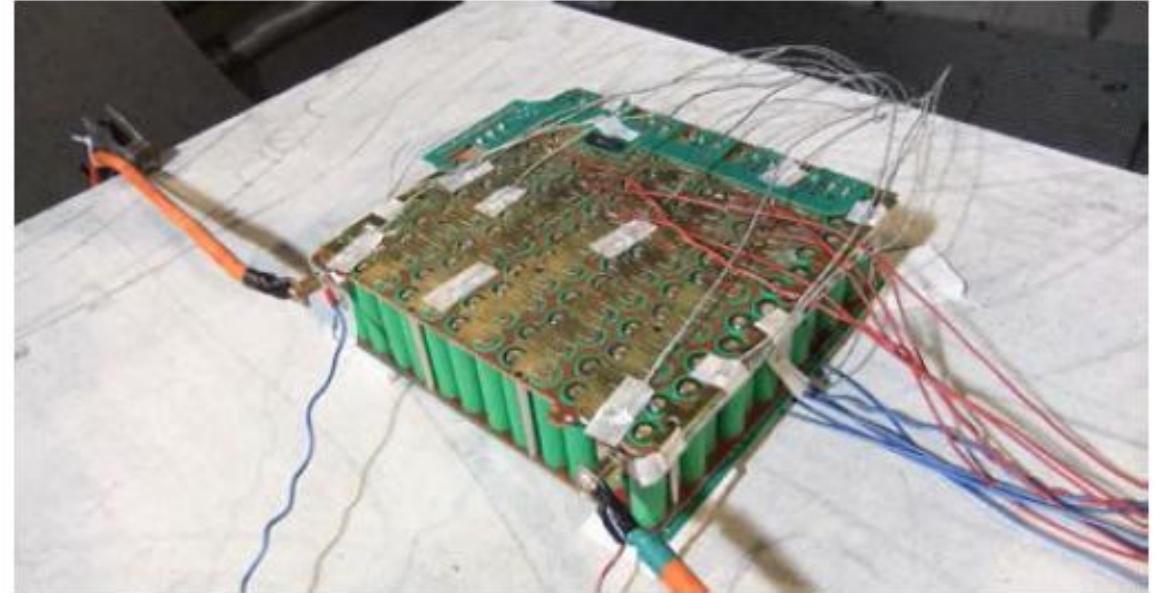
Module at test place after short circuit
