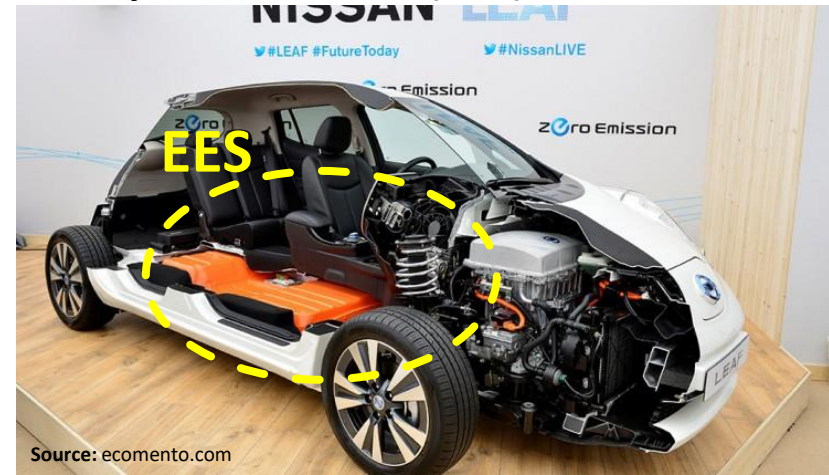
Battery installed in the (safe) center of the car
