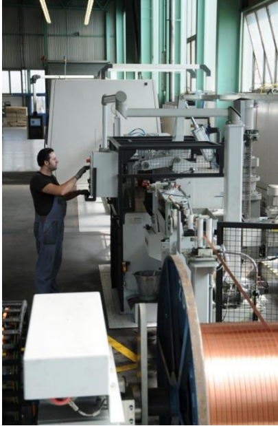
Fully automated rotor-bar production line with machining centre
