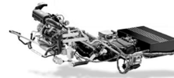
2010: Underfloor package 206 g Platinum 4 kW / m 2 active area Screw compressor
