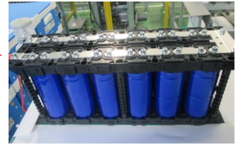
Figure 3: Electrochemical capacitor module used to power the AGV. Twelve model DXE 3600-F Nippon Chemi-Con electrochemical capacitors are connected in series. The module is rated at 30 V and can deliver ~100 kJ (28 Wh) with discharge to 15 V.
