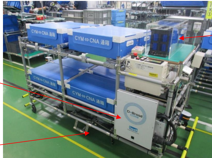
Figure2. Photograph of capacitor-powered AGV located at the Nippon Chemi-Con factory in Nagaoka, Japan.
