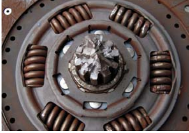
Figure 1: A broken shaft in the clutch
