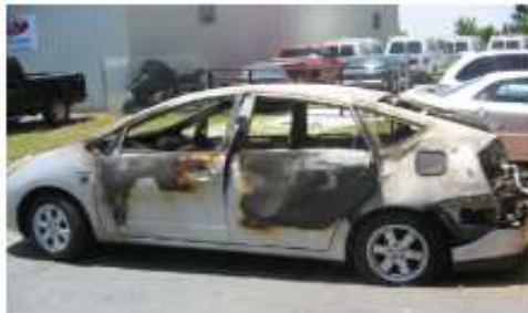
Fire in Prius Plug-in Origin : incorrect tightening of a nut on electrical connection
