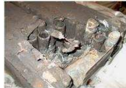
Damaged connections in a Prius Plug-in
