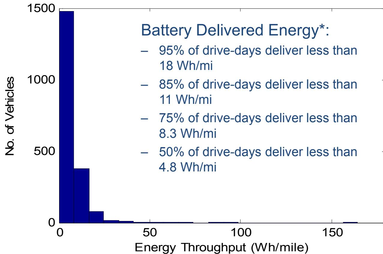
*\*Delivered Energy = sum of all battery discharges (includes both engine start and aux load discharges)*
