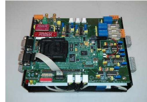
Monitoring and diagnostic platform for electric
