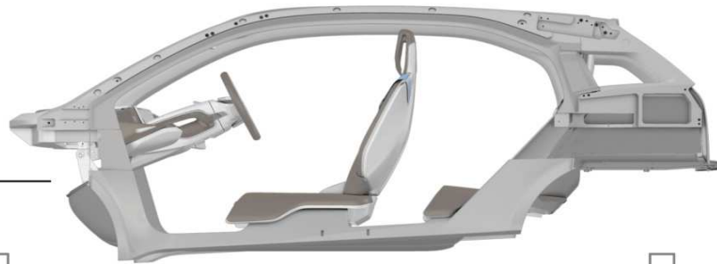
Life-Modul with CFRP passenger compartment
