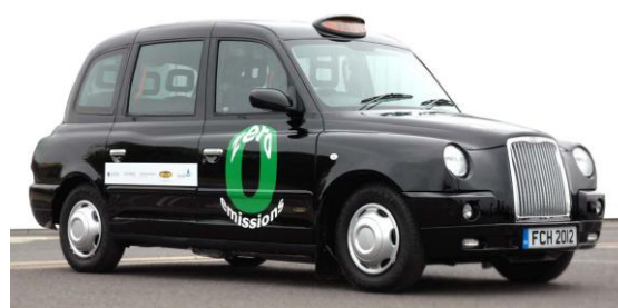
Figure 5: Prototype Fuel Cell Hybrid Taxi
