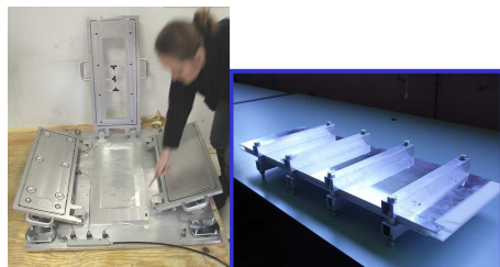
Figure 3: Mechanical assembling tool (left) and tightening plates (right) for bipolar cells prototyping.
