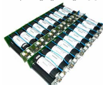
Figure 6: 2nd generation SAM with 40 SCAPs: the multilayer PCB contains the main current conductors, the patented balancing circuitry VP (virtual parallel circuit), supervision as well as a CAN-bus interface
