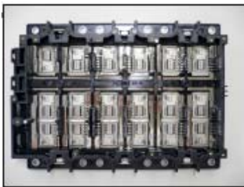
The 2 nd generation Power module for generator/motor
